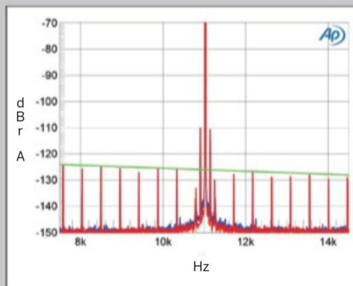
**Fig.16** Métronome c|AQWO, high-resolution jitter spectrum of analog output signal, 11.025kHz at -6dBFS, sampled at 44.1kHz with LSB toggled at 229Hz: 16-bit USB data (left channel blue, right red). Center frequency of trace, 11.025kHz; frequency range, ±3.5kHz.
