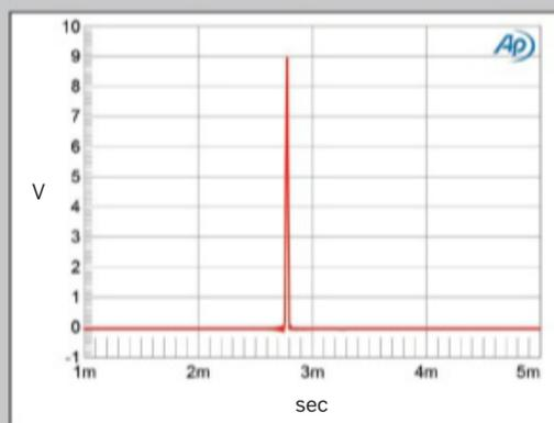
**Fig.1** Métronome c|AQWO, Super Slow Roll-Off filter, impulse response (one sample at 0dBFS, 44.1kHz sampling, 4ms time window).
