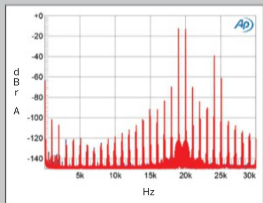
**Fig.14** Métronome c|AQWO, solid-state output, Low Dispersion Short Delay filter, HF intermodulation spectrum, DC-30kHz, 19+20kHz at 0dBFS into 100k ohms, 44.1kHz data (left channel blue, right red; linear frequency scale).
