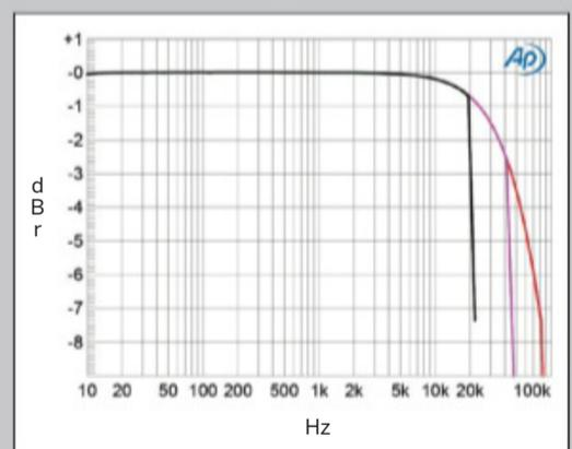
**Fig.8** Métronome c|AQWO, Sharp Roll-Off filter, frequency response at -12dBFS into 100k ohms with data sampled at: 44.1kHz (left channel green, right gray), 96kHz (left channel cyan, right magenta), 192kHz (left blue, right red) (1dB/vertical div.).
