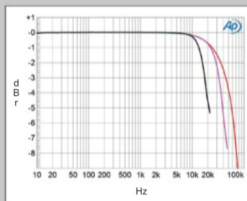
**Fig.7** Métronome c|AQWO, Slow Roll-Off filter, frequency response at -12dBFS into 100k ohms with data sampled at: 44.1kHz (left channel green, right gray), 96kHz (left channel cyan, right magenta), 192kHz (left blue, right red) (1dB/vertical div.).
