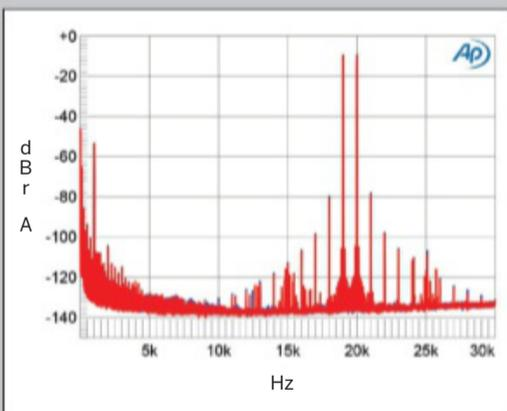
**Fig.15** Métronome c|AQWO, tube output, Sharp Roll-Off filter, HF intermodulation spectrum, DC-30kHz, 19+20kHz at -6dBFS into 100k ohms, 44.1kHz data (left channel blue, right red; linear frequency scale).
