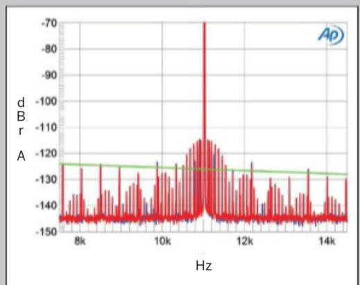
**Fig.17** Métronome c|AQWO, high-resolution jitter spectrum of analog output signal, 11.025kHz at -6dBFS, sampled at 44.1kHz with LSB toggled at 229Hz: 16-bit TosLink data (left channel blue, right red). Center frequency of trace, 11.025kHz; frequency range, ±3.5kHz.
