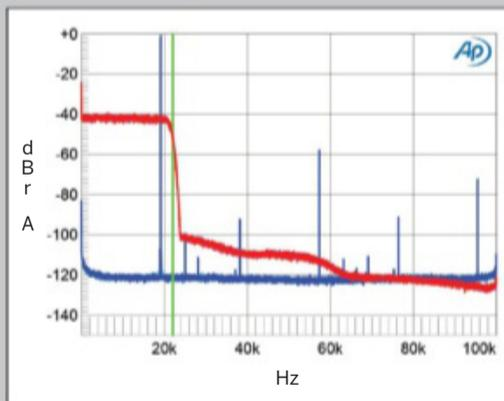
**Fig.4** Métronome c|AQWO, Sharp Roll-Off filter, wideband spectrum of white noise at -4dBFS (left channel red, right magenta) and 19.1kHz tone at 0dBFS (left blue, right cyan) into 100k ohms with data sampled at 44.1kHz (20dB/vertical div.).
