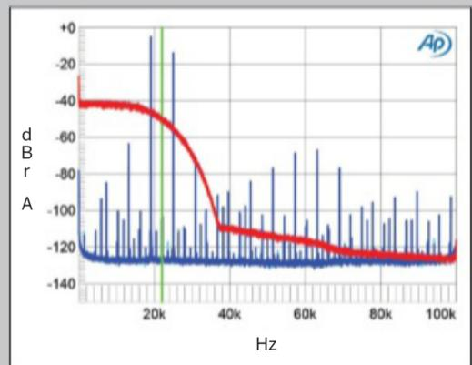
**Fig.5** Métronome c|AQWO, Slow Roll-Off filter, wideband spectrum of white noise at -4dBFS (left channel red, right magenta) and 19.1kHz tone at 0dBFS (left blue, right cyan) into 100k ohms with data sampled at 44.1kHz (20dB/vertical div.).
