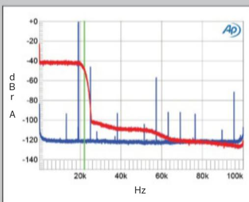
**Fig.6** Métronome c|AQWO, Low Dispersion Short Delay filter, wideband spectrum of white noise at -4dBFS (left channel red, right magenta) and 19.1kHz tone at 0dBFS (left blue, right cyan) into 100k ohms with data sampled at 44.1kHz (20dB/vertical div.).
